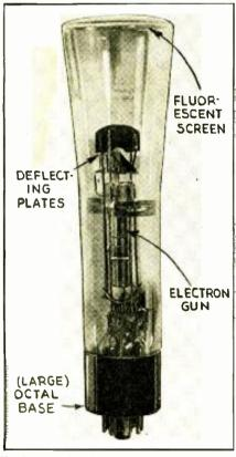
Fig. 8. The 24 XH high-vacuum cathode-ray tube is very similar in construction to its larger brother the 34 XH (906), with the exception that it focuses to a screen closer to the deflecting plates. This calls for a change in the shape of the deflecting plates. The area of the screen of this tube is 4 times that of the 913 or 1-in. C.-R. tube which increases its usefulness many times over the (latter) small tube. The 2nd. anode operates at 600 V. (max.).
